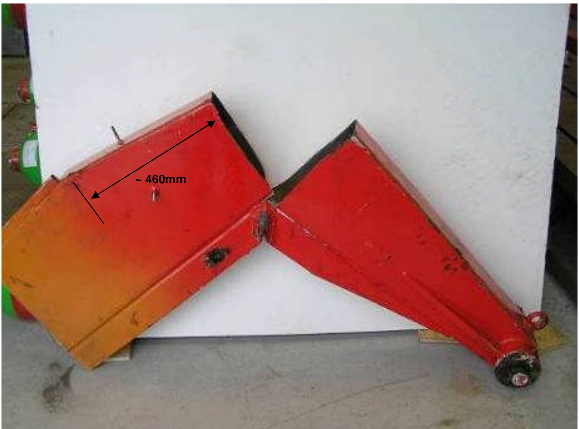
P8040173 – Failed Arm Photographed at HSL
