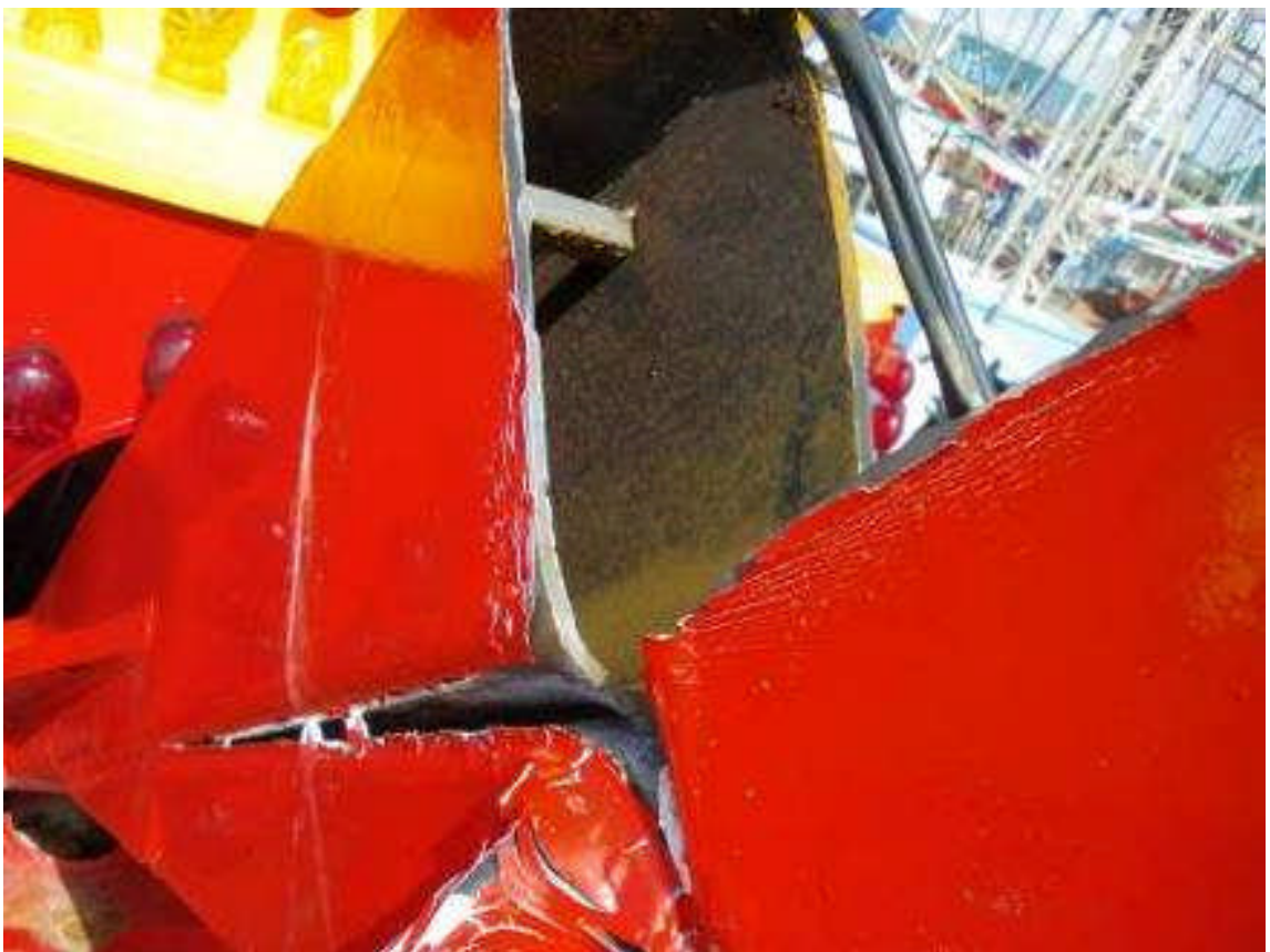
IMGP1561 – Failed Arm
