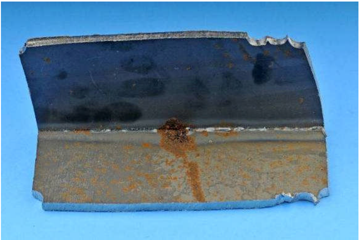
Fig.05 – Internal View of Cracked Arm
