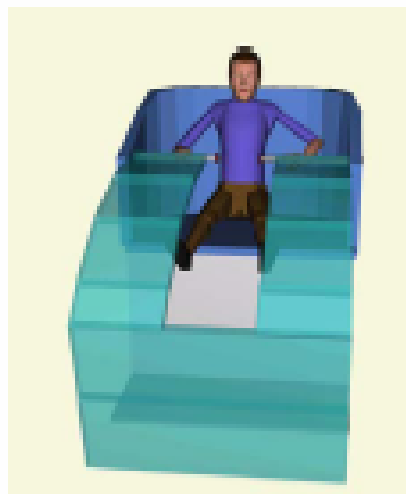
Figure 8. JACK Illustration of a 50 th percentile 7 year old boy on the Octopus. A central gap between the two sides of the handrail, measuring 175mm is illustrated.
